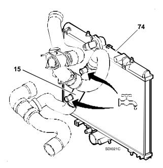
15 - air/water heat exchanger (inlet air heater)
