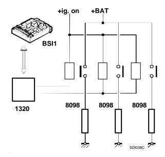
Assembly with 3 relays and 3 resistors
