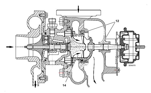
The gas flow passing through the exhaust turbine (14) is low.
