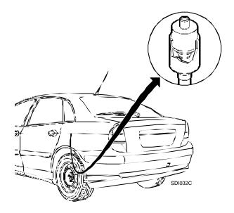
The safety valve is located in the rear left hand wheel arch (behind the mud flap).
