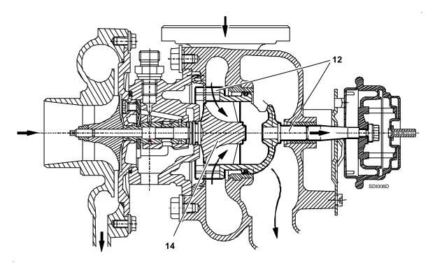
Turbocharging pressure regulation: the energy of the exhaust gases is controlled by adjusting the speed at which the gases enter the exhaust turbine by altering the position of the finned diffuser piston.
