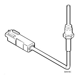
The sensor consists of a Negative Temperature Coefficient resistor (NTC).
