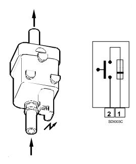
The fuel heater heats the fuel from the fuel tank.
