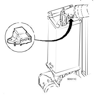
The inlet manifold pressure sensor is located on the outlet of the air/air heat exchanger.
