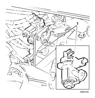
The electrovalve is located in the engine compartment.
